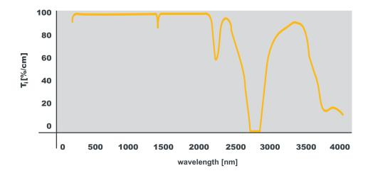
HPFS® Standard Grade is certified to meet T external  $\geq 80\%$ /cm @185nm (T internal  $\geq 88\%$ /cm @185nm), when measured through a polished, uncoated sample.
