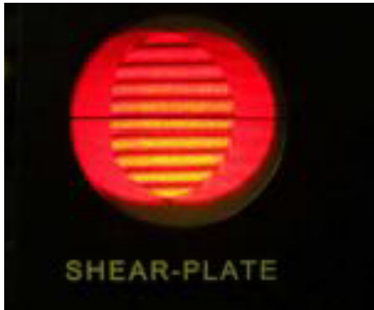
Figure 3: Shear plate interferogram for a collimated beam
